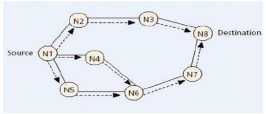
Fig.1.Path Discovery in AODV (Deng et al. 2002)
